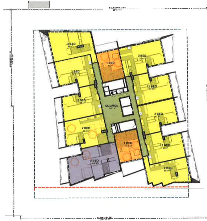
Apartment Mix: Level 2-6 SCALE 1:307.69 @ A1
